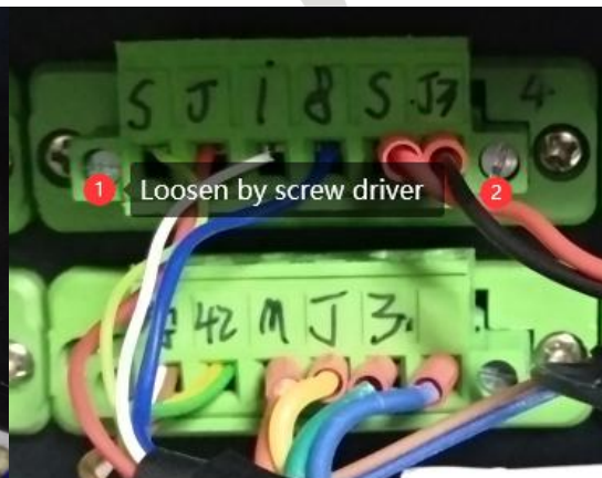
Two screws on green cable need to loosen (1)
