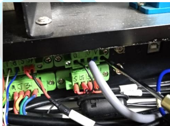
Two screws on green cable need to loosen (2)
